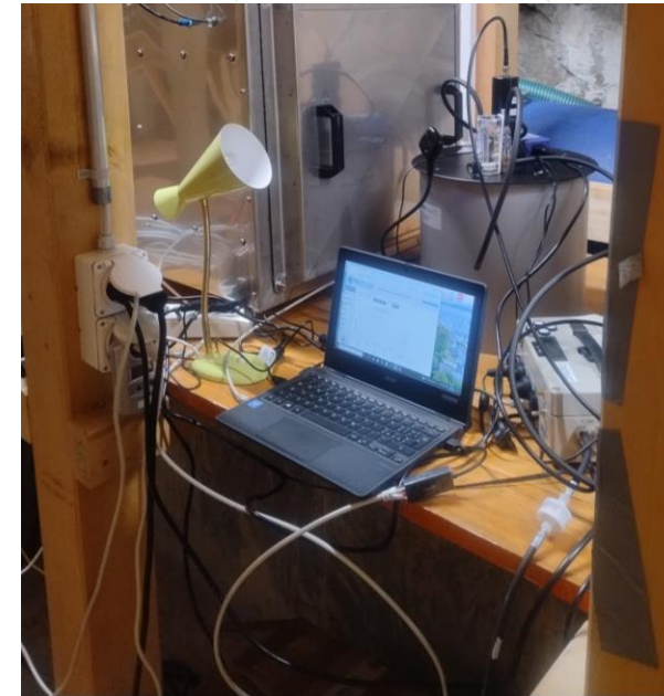
Radon detector of ISAC – CNR: Pylon detector (TEL model) coupled with Radon Mapper Monitor of Tecnavia/Mi.am (Italy).
