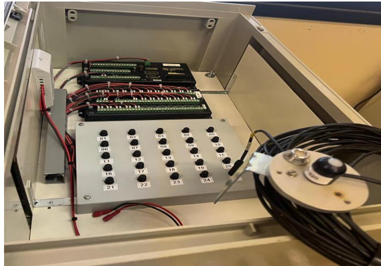
Quantum sensors installed in Castelporziano (Campo di Rota), and the greenhouse at Tuscia University
