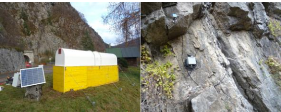
Monitoring system: GB-Insar has been installed, in November 2024, and every 1 h it captures an interferogram
