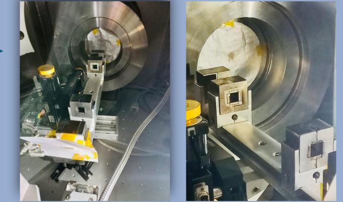
With the MBL the point size is reduced from  $1.15 \times 0.90$  cm to  $0.60 \times 0.44$  cm, whereas the point stability deviation is reduced from 1.99 to 0.55 and from 2.81 to 0.44, for  $\sigma_x$  and  $\sigma_y$ , respectively.
