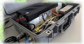
The  $LI-78\,10~(\mathrm{CO_2},\,\mathrm{CH_4},\,\mathrm{and}\,\,\mathrm{H_2O}$  analyzer) enables high-precision, long-term monitoring of greenhouse gas emissions and can be mounted on a backpack for real-time field data acquisition in both static and dynamic configurations. The instrument supports soil experiment measurements, and up to 16 units can be interconnected to continuously monitor  $\mathrm{CO_2},\,\mathrm{CH_4},\,\mathrm{and}\,\,\mathrm{H_2O}$  emission rates across larger areas.
