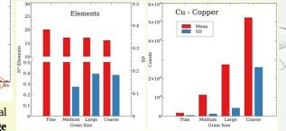
The XRF technique combined with the EDXRF detector has proven to be highly effective, allowing rapid and simultaneous identification of elements within the sample. Granulometric analysis indicated that the fine fraction is optimal for identifying elements in the ground sample. Conversely, larger particle sizes, despite offering a higher signal-to-noise ratio, introduced greater variability into the measurements.
