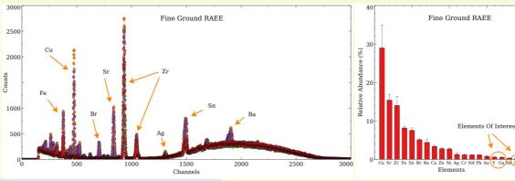
**Results & Conclusions** As expected, larger particle size reduces the ability to identify **Elements**, increasing variability between samples. Furthermore, while signal intensity (counts) of the identified elements increases (**Mean**, **Cu-Copper**), so does the variability of the mean value (**SD, Cu-Copper**) across all samples of the same granulometric size
