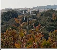
The CO<sub>2</sub> and H<sub>2</sub>0 exchange are monitored with an eddy covariance system.
