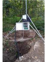
Soil environmental conditions and CO<sub>2</sub> fluxes are monitored continuously
